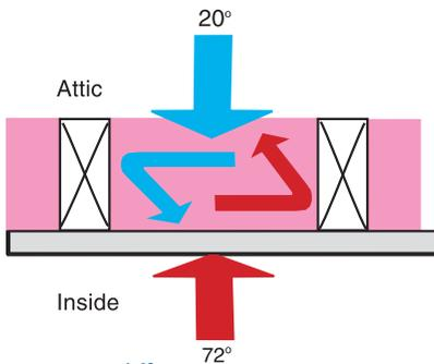
Dramatic differences in air temperature create convective loops in fiberglass insulation. Because of its density, Nu-Wool Premium Cellulose Insulation reduces convective loops and the resulting heat loss.
